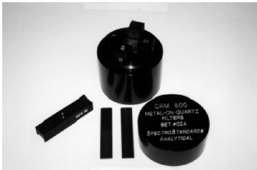
Figure 3. The SpectroStandards™ CRM 500 neutral-density metal-on-quartz filter set. CRM 500 consists of three individual filters in separate metallic cuvette-style holders and one empty filter holder. The nominal percent transmittances of the three filters are 10%T, 30%T and 90%T. The filter holders are provided with removable sliding shutters that are intended to protect the filters when not in use. Each filter holder is engraved with a unique filter number (10, 30 or 90) and a set identification number. The filters are stored and transported in a cylindrical canister.
