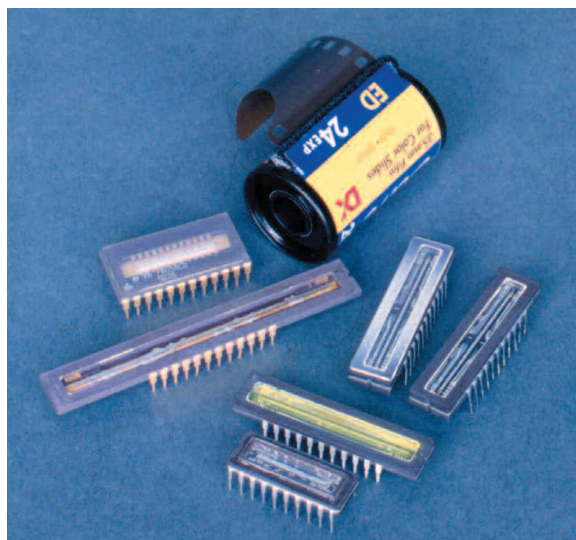
Figure 1 The relative size of linear CCDs arrays used in spectroscopy applications is contrasted against the roll of film they have come to replace in recent years.
